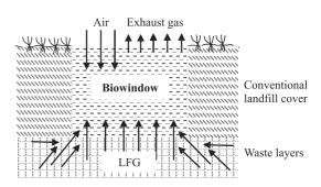
Fig. 4: Conceptual scheme of biowindows. LFG, landfill gas.
