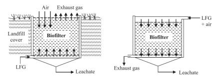
Fig. 3: Variants of biofilter design. Left: up-flow biofilter integrated into landfill cover: right: biofilter in down-flow mode. LFG, landfill gas.
