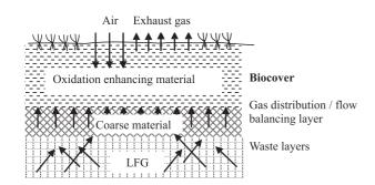
Fig. 2: Conceptual scheme of a biocover. LFG, landfill gas.
