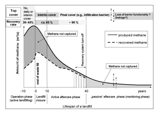
Fig. 1: Time-dependent methane production and recovery over a landfill lifetime. Methane emissions (methane not captured) are shown as a function of cover type and do not include methane oxidation removal: gas recovery rates according to Spokas *et al.* (2006) and (Huber-Humer 2007).
