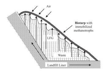
Fig. 5: Conceptual scheme of biotarps. LFG, landfill gas.
